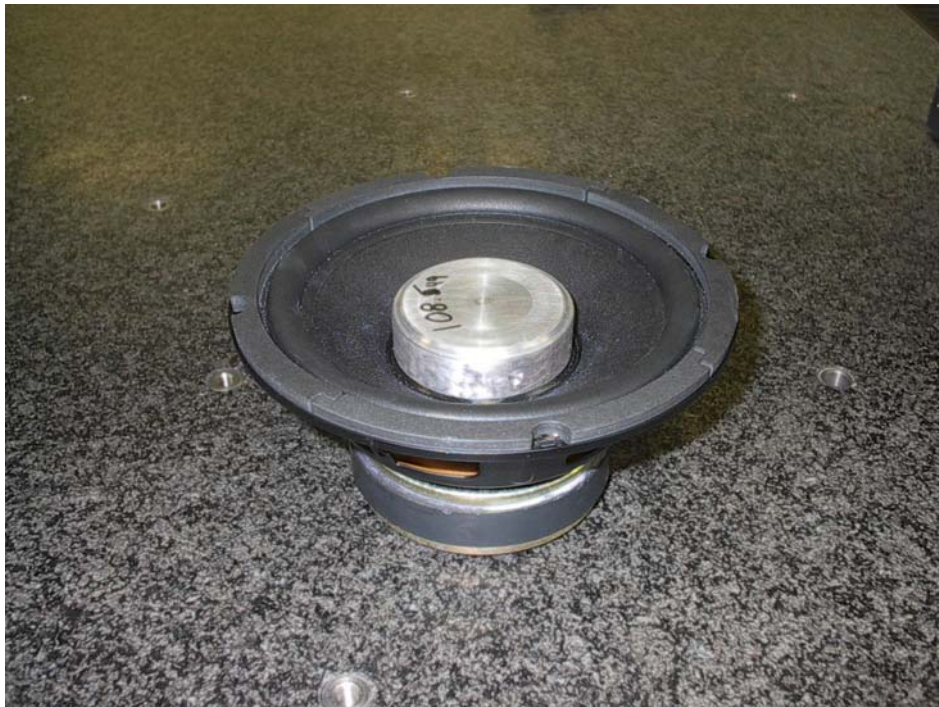
Fig. 2.3. Photograph of the aluminum cylinder placed on the driver under test. The cylinder provided an even load distribution to the driver diaphragm.
