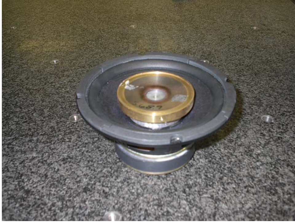
Fig. 2.4. Photograph of an additional known weight, which results in a measurable displacement using the CMM. The added weight contains a hollow center allowing a point of reference to be maintained.
