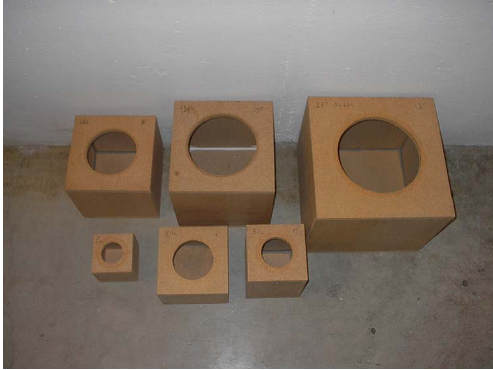
Fig. 4.6. Photograph of various test boxes used for closed box perturbation tests.
