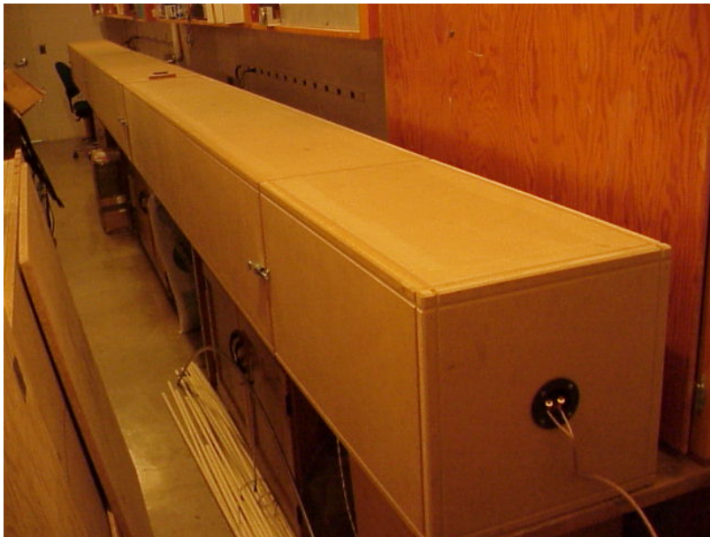
Fig. 5.5. Photograph of the entire constructed plane wave tube. View is arranged with the excitation source in the forefront and with the termination at the far end.
